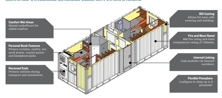
HB Rentals' 32' DNV A60 Linkable Sleeper can accommodate up to 8 individuals. Certified to DNV 2.7-1, the 32' sleeper module is designed to maximize worker safety and comfort. Versatile in its design, the module provides the comforts of home and easy plug and play connections with safe and quick installation features. Clever engineering allow our modules to link horizontally and stack up to four units high.
